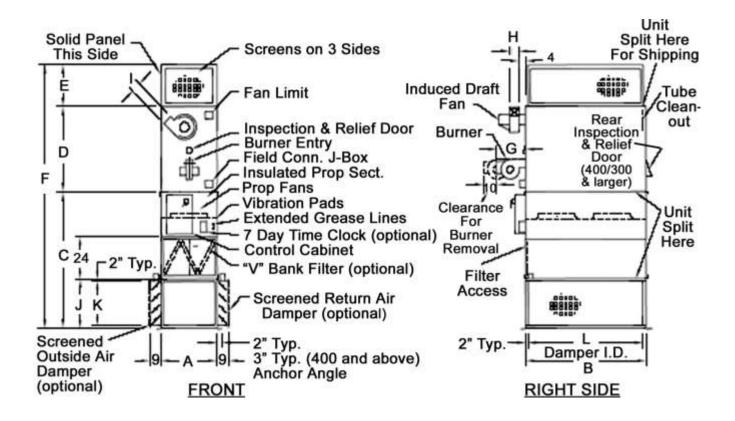
**NOTE:** On units 200 and above discharge section is shipped knocked down (field assembly by others).
