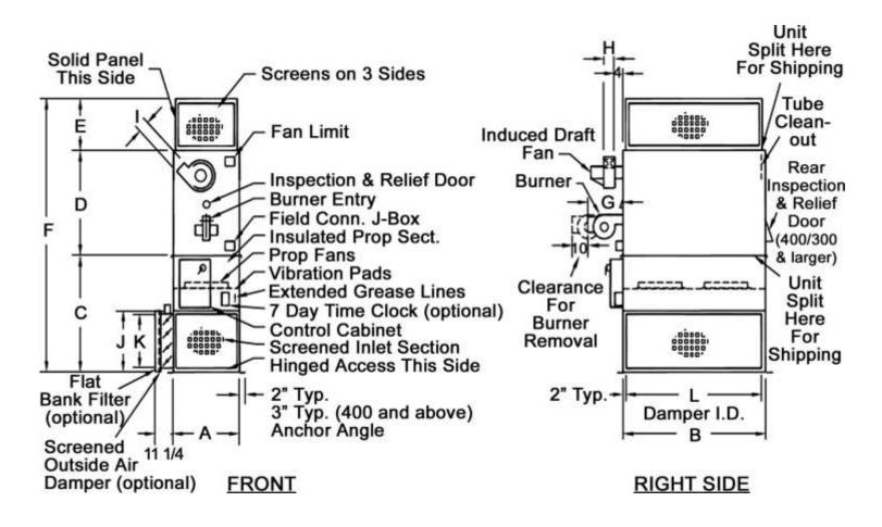
**NOTE**: On units 200 and above discharge section is shipped knockdown (field assembly by others)
